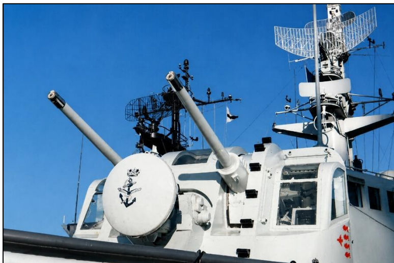
The 3" Anti-Aircraft Gun and Fire Control Radar I Maintained
